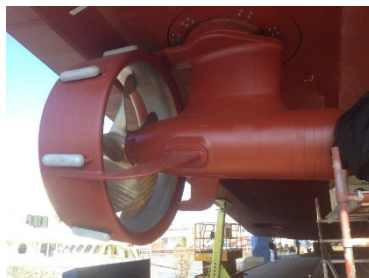
V-POD propulsion system
